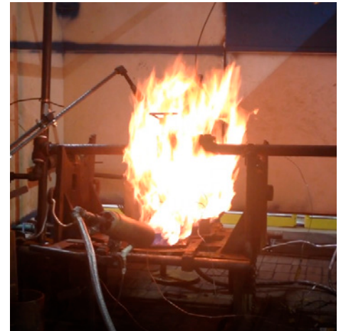
Fire test per API Spec 607 4th Edition.
