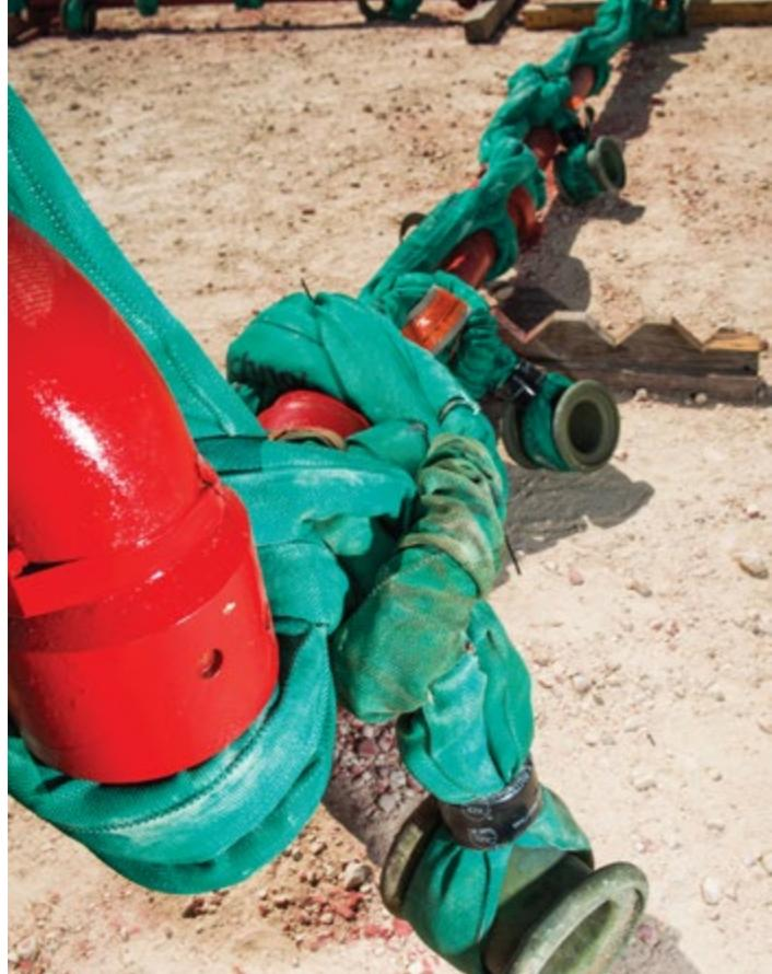
TechnipFMC's Temporary Pipe Restraint (TPR) system is used on high pressure temporary flowlines. Properly applied, this system will provide an additional level of protection for personnel and physical assets by minimizing the amount of sudden movement in the event of an iron failure. The TPR system comes in two models: Standard and Premium.
